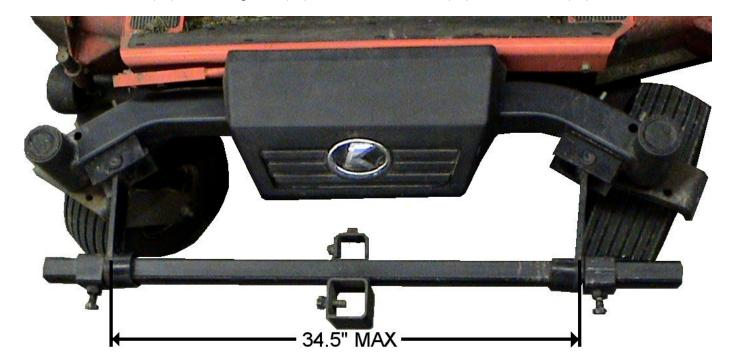
Step 3. Place side supports (06) into front brackets (08). Secure with connector pins (19) and linch pins (26).
