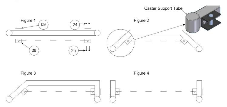
Step 2. Secure front brackets (08) and back plates (09) as shown. Use bolts (24) and lock nuts (25).
