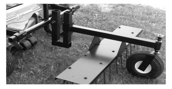
Insert the "U" shaped tube into the universal mount bar and hand tighten. Insert the dethatcher onto the "U" shaped tube as shown and hand tighten.
