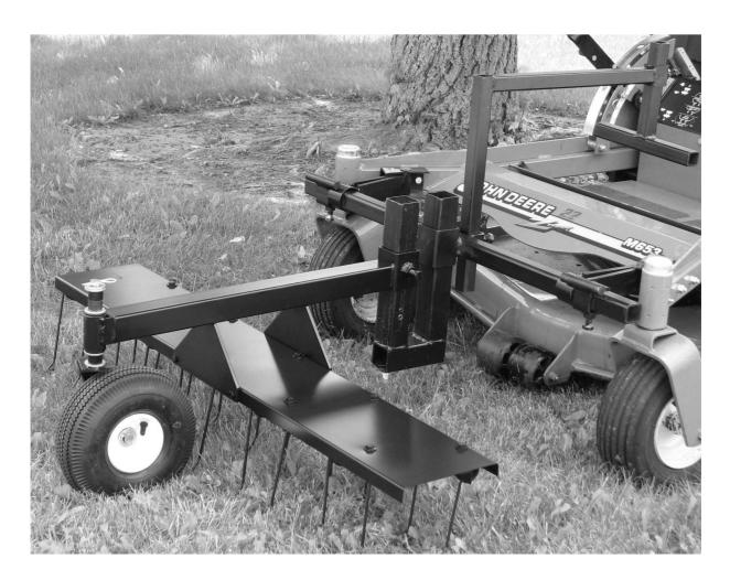
Adjust the unit so that the main support is level with the ground and tighten the bolts on the "U" shaped tube. You will also need to adjust the height of the front tire using a combination of spacers and 3/4" flat washers. Insert the foot pedal assembly and adjust the height as needed. You will use the foot pedal to lift the dethatcher for transport.
