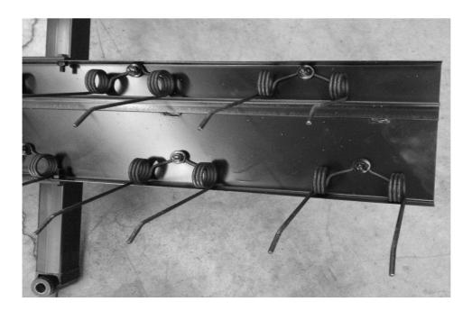
Attach 12 tines to the plate as shown. Use 1 - 5/16" x 1" bolt / nut and 2 - 5/16" washers. (Please note the direction of the tines and position of the plate. These will only bolt together one way.)
