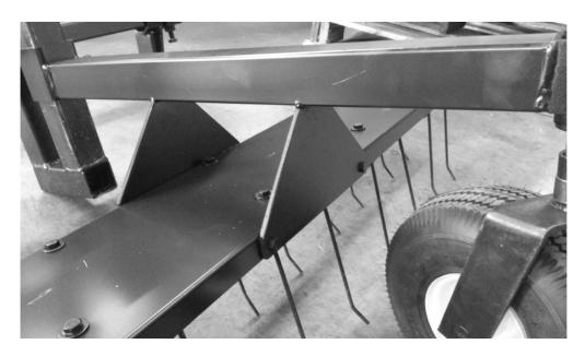
Attach the main support tube to the mounting plate using  $4-5/16" \times 1"$  bolt / washer / lockwasher / nut. Make sure the tines are facing towards the front of the support tube as shown.
