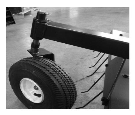
Insert the axle assembly into the main support with a 3/4" flat washer on each side of the bearing tube. Place 3 spacers on the upright shaft and use the quick release pin to hold in place. The spacers and 7 - 3/4" washers will be used to adjust dethatching depth. Attach the tire using 1 - 3/4" washer and 1/8" cotter pin. Make sure the valve stem is facing outward as shown above.
